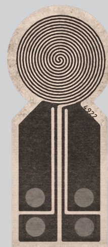
Mica-insulated Hot Disk ® sensors
